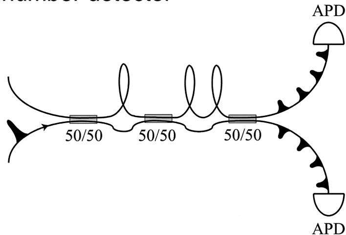
Fiber-assisted detection with photon number resolution,
