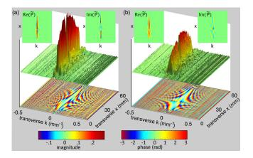
FIG. 2 (color online). Directly measured Dirac distributions for (a) pure and (b) mixed states. In both (a) and (b), the left and right insets are the directly measured real and imaginary parts of the Dirac distribution  $\tilde{\mathbb{P}}(x, p)$ . From these, we calculate the magnitude (upper plot) and phase (lower plot) of the distribution. Transverse *x* corresponds to the position of the quartz sliver (i.e.,  $|x\rangle\langle x|$ ); transverse  $k = p/\hbar$  is the transverse wave vector.
